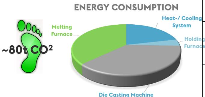
Figure 9: Energy consumption of high pressure die casting process [9]
