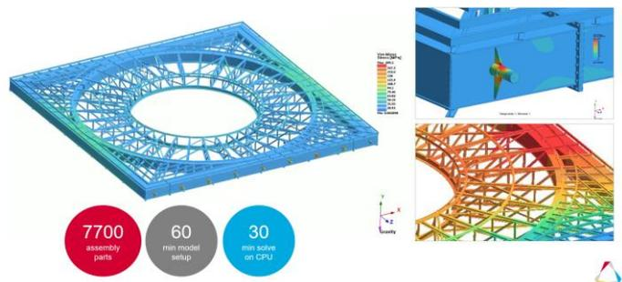
This structure has over 7700 parts, model import and setup were made in 60 minutes and the solving part was done on 30 min, on a normal computer.
