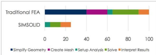
The second benefit is expanding the possibilities of what is practical to solve. Instead of reducing the assembly to one part or a small context of a few parts, a more complete assembly can be solved, simplifying the model setup and load and constraint specification. Many models that are not practical to use with traditional FEA can be solved using SimSolid.
